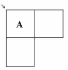
The bottom panels have velcro on top, springs on bottom. Start in <u>one</u> corner with three bottom (springed) 5' x 5' panels. (Do not start at each corner and work toward center.) Carefully align the edges to be squared up.
