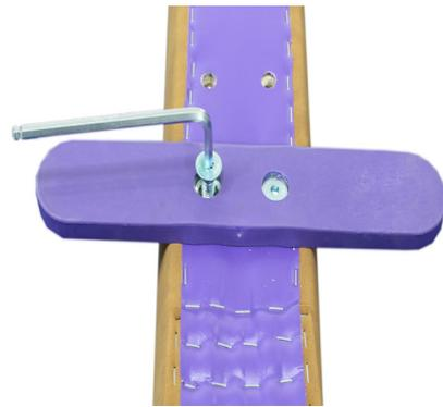
3. To reattach the outer feet, place one end spacer (F) on the outer screw holes. Place the foot onto the spacer, aligning the screw holes.
