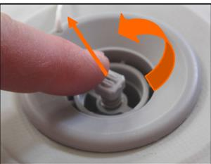
To CLOSE: Push down and turn on the gray button. It should pop back up. Use this position when using hand pumps to fill, or to top off the pressure after the electric pump.
