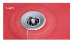
STEP 2 – Before inflating make sure the valve is closed. To close valve push the pin down and turn a quarter of the way around. The pin should be slightly taller than the rim of the valve. Connect the adapter to the hand pump tube after removing the Green Ring (leaving the yellow and black ring). Insert the adapter into the valve by pushing down and turning clockwise to lock in place. Start using the pump to inflate. Put the dust cover on once inflated.
