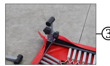
Insert the longer Mini Trak foot in the extension making sure the holes line up with the D-2 spring knob holes. Attach the D-1 knobs in the lower hole facing the front of the Mini Trak and tighten to secure the extension. Insert the longer D-2 spring knob in the holes facing each other and turn till tight. You will then be able to loosen and pull on the knob to allow the legs to slide up and down to change the height.
