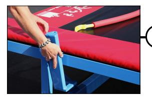
Slide Bracket #1 into position, placing it tightly against the leg. Close the hinge and replace the PTO pin into the hole on the "U" (hook) part of the bracket. Locate the leg of your Tumbl Trak on which you want to place the Quick Flex Bar bracket. Remove the PTO pin of Bracket #1 and open the hinged portion of the bracket.
