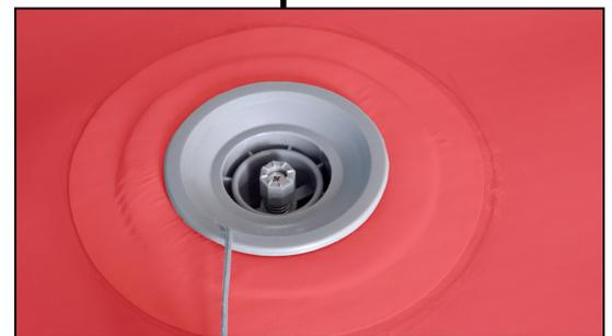
**STEP 3** – To open the valve and deflate the Air Pit push the pin down and turn a quarter of the way around. The pin should sit just below the valve rim.
