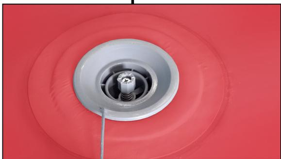
**STEP 2** – Before inflating make sure the valve is closed. To close valve push the pin down and turn a quarter of the way around. The pin should be slightly taller than the rim of the valve. Connect the adapter to the black cone nozzle. Insert black cone nozzle and adapter onto electric pump. Insert it into the valve by pushing down and turning clockwise to lock in place. Turn the pump on to inflate. Put the dust cover on once inflated.
